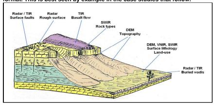
Impact of surface features on seismic survey logistics and data quality. Surface features often encountered in land seismic surveys can be discriminated using combinations of spectral bands (table, *below*). An example from a desert environment illustrates some of these features (sketch, *above*).
