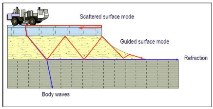
Surface modes in seismic acquisition. Seismic energy from a vibrator truck is directed to deep formations as body waves. However, significant energy is scattered or trapped near the surface. Rayleigh waves travel along the surface and can scatter from escarpments or at changes in lithology. Other seismic energy can be trapped in soft sediments between harder layers, or can be refracted at the interface.
