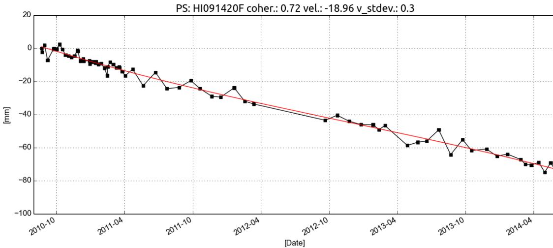
***Figure. The temporal evolutions (black lines) and the corresponding second degree polynomial regressions (red lines) for a point on the ground located in the Southern exit of the railway tunnel in the Mamayka area. The analysis covers the period August 2010 - May 2014***
