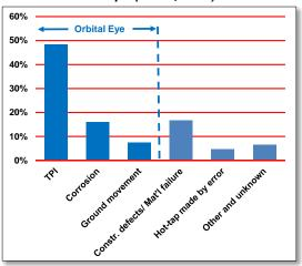
Figure 2: Causes for pipeline failures in USA (PHMSA<sup>iii</sup>, 2011)
