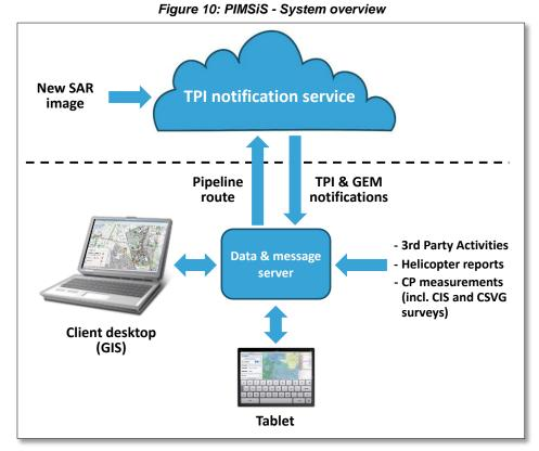
Orbital Eye's desktop & tablet system supports a GIS application which can manage the following object and display their locations on a geographic map:
