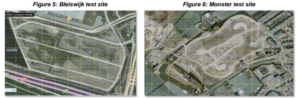
The Bleiswijk test site is an area planned for industrial development but, due to the financial crisis in 2013, without any building activity. The soil of this test site is peat and clay. The Monster test site is an area for urban development, but for the same reason also without any construction activity. The soil of this test site is sand.
