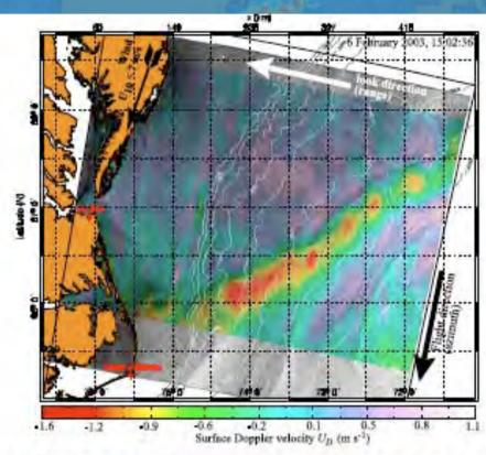
Figure 1. Normalized mater cross-section  $\sigma_0$  (gray shades) and Doppler velocity  $U_D$  (colors), analyzed from a wide-swath image obtained by ENVISAT on 6 February 2003 at 1512 UTC. Oceanic fronts appear as sharp gradients of  $\sigma_0$ , while the surface velocity seen by the radar appears to be related to the Gulf Stream.
