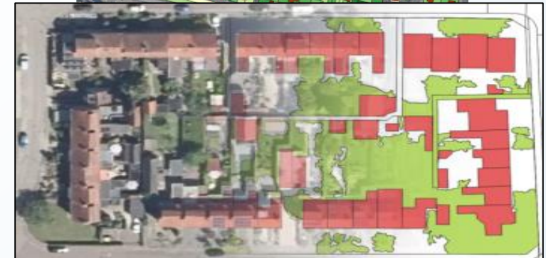
Surface sealing area
