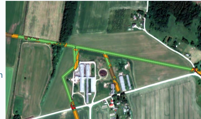
Water leakage risk detection
