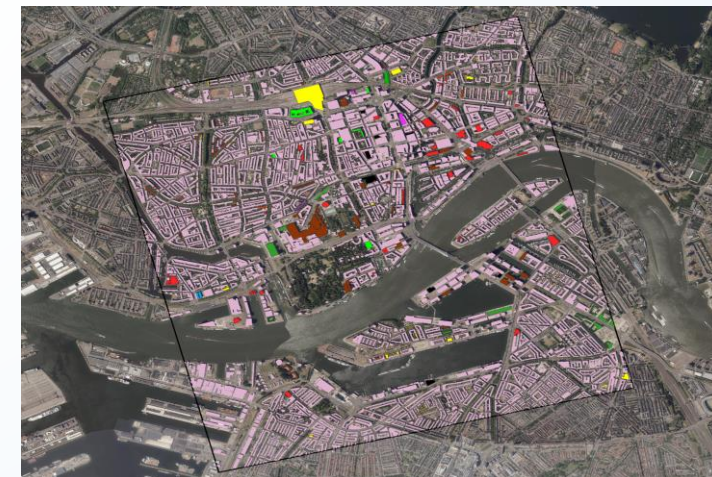
Detected roof types of Rotterdam overlaid on an RGB image
