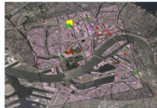
Detected roof types of Rotterdam overlaid on an RGB image
