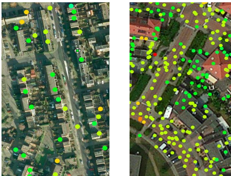
Figure 4-1: InSAR measurement point density of standard resolution images (Envisat, left) and very high resolution images (TerraSAR-X, right) (courtesy SkyGeo).
