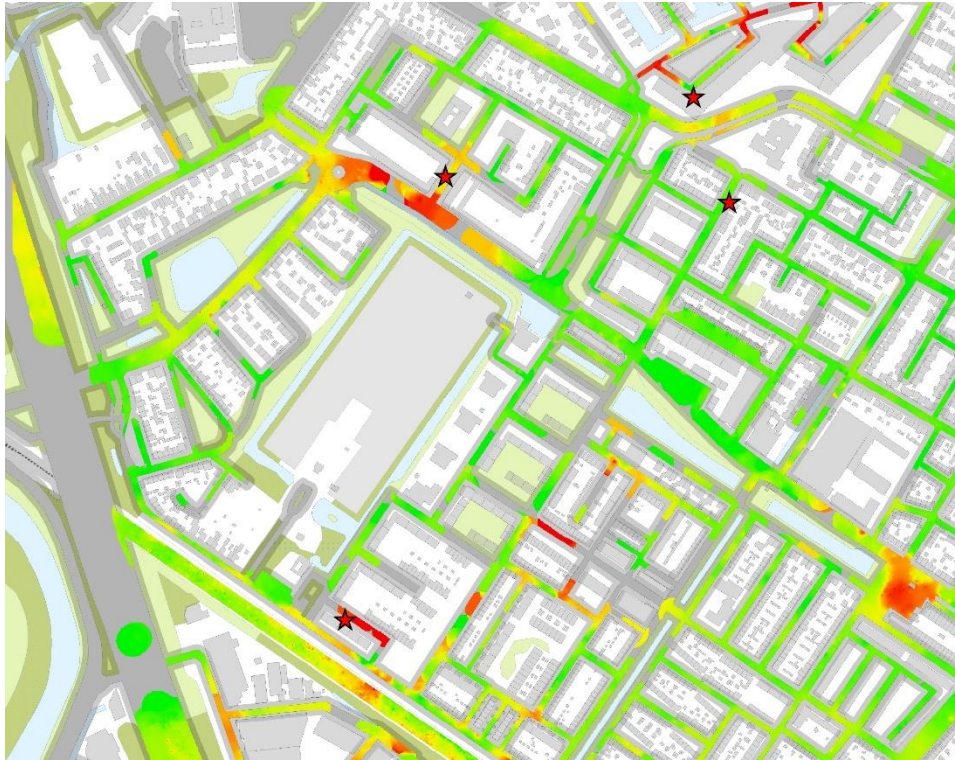
Figure 2-9: Heat map used by Oasen showing ground movement mapped along the streets carrying pipelines. (courtesy SkyGeo)
