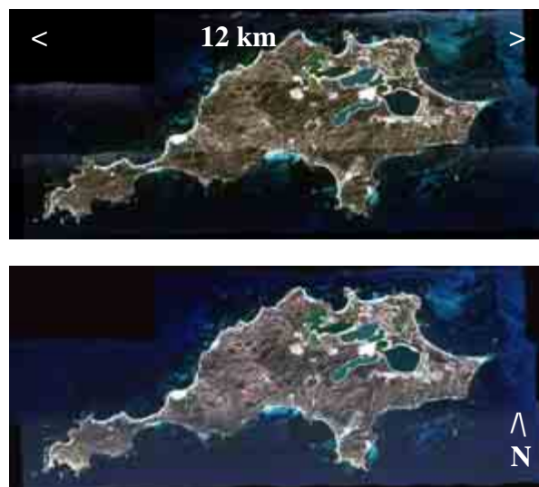
Figure 2 HyMap 'true' colour composites – top: uncorrected bottom: corrected for sun glint over water and BRDF effects over land
