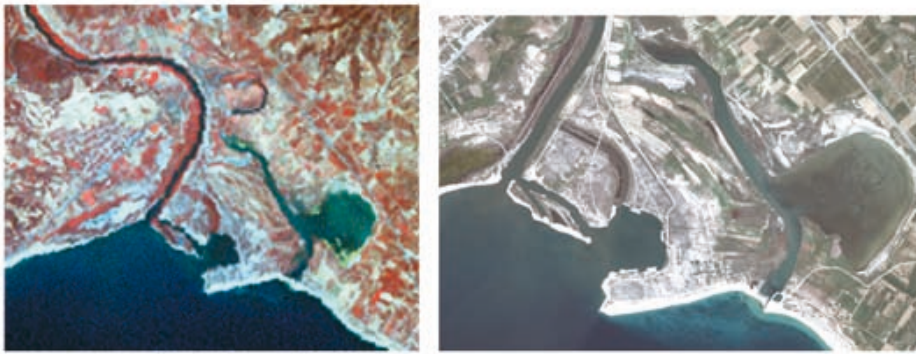
Figure 2.14. The satellite images show the delta of River Strymon in Northern Greece. The image on the left is a Landsat ETM+ with spatial resolution of 30 m. On the right, there is a subset of the same area as acquired by QuickBird satellite with a spatial resolution of 60 cm (Source: QuickBird© Digital GlobeTM Longmont USA).
