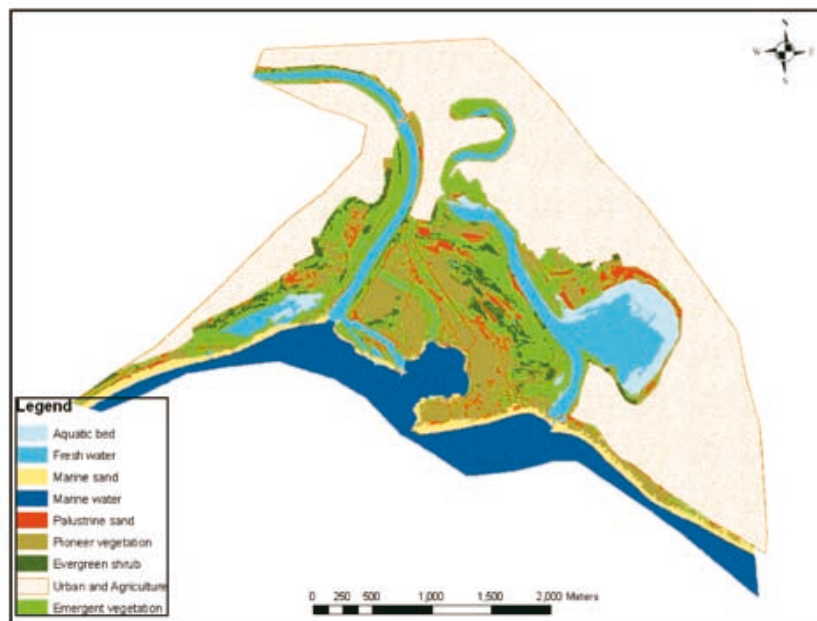
Figure 3.50. Classification result for the Strymon Study Area using the Nearest Neighbour Classifier and 200 scale parameter.
