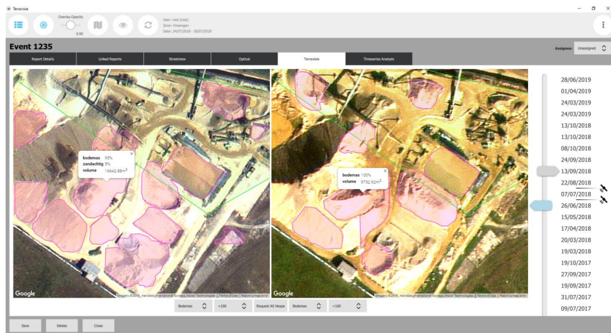
Bulk waste material monitoring tool estimating volumes and material class
