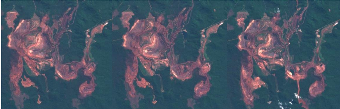
Caption Observation in time (July 2016, 2017 and 2019) of mining and rehabilitation activities at the Carajas mine, Brazil, with the help of Sentinel-2 images (source: Sentinel Hub).
