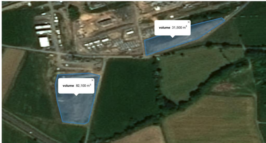
Figure 3-2: Example of an optical image with detected stockpiles and their estimated volume.
