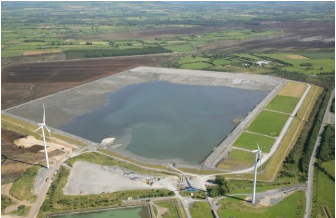
Figure 26 – Lisheen Mine – Tailings Management Facility 2014 – Progressive rehabilitation started
