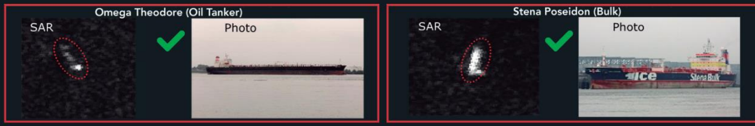
Example of ship detection and categorization from SHIP MONITORING SUITE (SIMON) project (Source: GMV)
