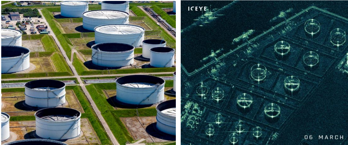
(Left) Oil tanks with floating roof (Right) Floating oil tank roofs in the Port of Rotterdam, Netherlands using ICEYE's Daily Coherent Ground Track Repeat (GTR) imagery (0.5 m) (Source: ICEYE).
