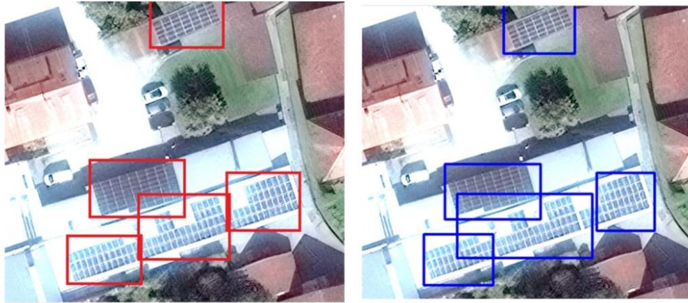
Ground truth for solar panels bounding boxes (Left) and prediction using deep learning-based object detection model (Right) using Worldview-3 images (0.3 m) over southern Germany (Source: Maxar).
