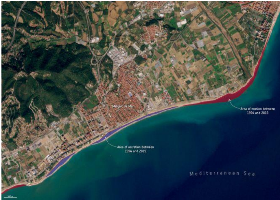
Shoreline changes along the coast of Malgrat de Mar, Spain. The 1994 coastline data is extracted from US Landsat data while the 2019 data is from the Copernicus Sentinel-2 mission. (Source: ESA).
