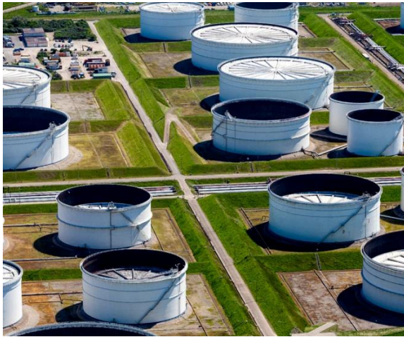
(Left) Oil tanks with floating roof (Right) Floating oil tank roofs in the Port of Rotterdam, Netherlands using ICEYE’s Daily Coherent Ground Track Repeat (GTR) imagery (0.5 m) (Source: ICEYE).
