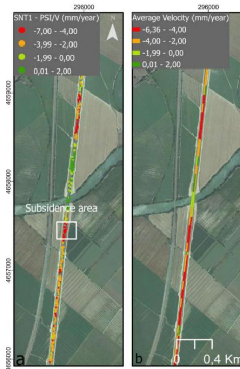
Displacement and average velocity maps PSI Sentinel-1 for D18 highway in Rome (Source: Orellana, F., Delgado Blasco, J.M., Foumelis, M., D'Aranno, P.J., Marsella, M.A. and Di Mascio, P., 2020. Dinsar for road infrastructure monitoring: Case study highway network of Rome metropolitan (Italy). Remote Sensing, 12(22), p.3697.).
