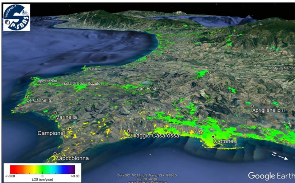
Google Earth output file obtained after P-SBAS InSAR processing of the 2014–2020 Sentinel-1 IW SAR ascending mode stack: detail over the area of Crotona province, southern Italy. (Source: Cigna, F. and Tapete, D., 2021. Sentinel-1 big data processing with P-SBAS InSAR in the geohazards exploitation platform: An experiment on coastal land subsidence and landslides in Italy. Remote Sensing, 13(5), p.885.).
